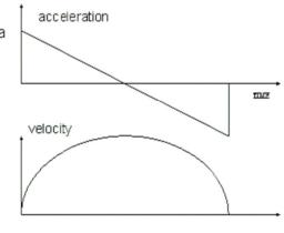
High currents at the ends saturates the Amp. Thus, parabolic profiles are not commonly used
